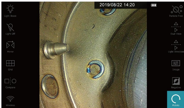
Rotate the live view clockwise to get the best visual angle
