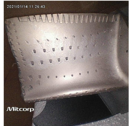
1600*1600 output by 3.9mm HD probe (30mm distance)
