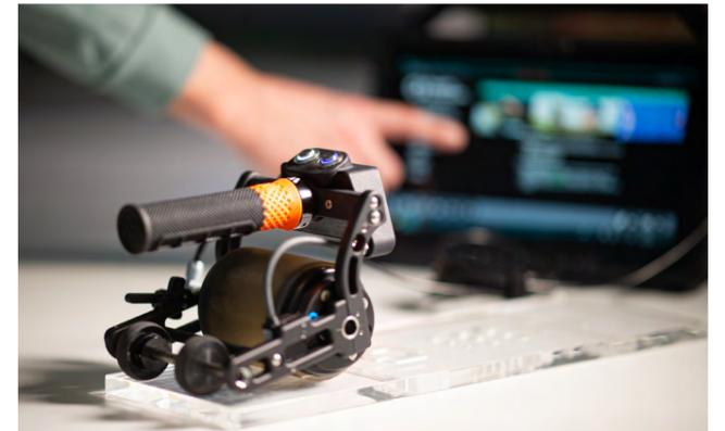
*Composite testing: inspection results are displayed on the tablet screen. Any Windows-based device can be connected to Krautkrämer RotoArray comPAct.*
