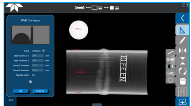
Wall thickness measurement
