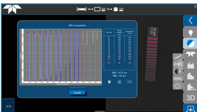
iSRb calculation and automatic IQI recognition
