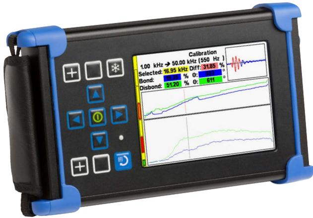
The BONDHECK is a multi-mode bond testing flaw detector. It provides high speed inspection in pitch-catch, resonance and MIA bond testing modes, with excellent defect sensitivity.
